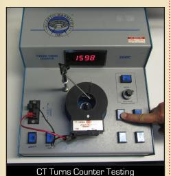
Utility Relay Company manufactures many of our CTs at our Chagrin Falls, Ohio facility. Each CT is ratio and polarity tested several times during production.
