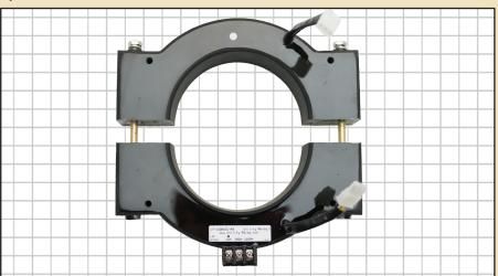
Utility Relay Company manufacturers split core CTs for use as neutral CTs in 4 wire systems. The split cores make it very easy to install the CT on existing bus or cable. Each split core has phenolic plates with punch outs to match standard sizes/shapes of cable or bus-work.
